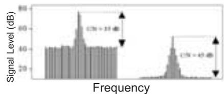
As can be seen in the illustration, it is not rare that a signal with a higher carrier level than another may have a lower C/N ratio, so this measurement is essential.
